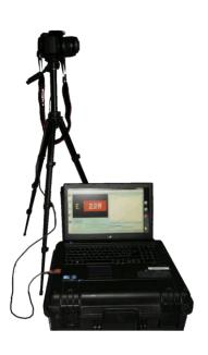
SMF/SIGN is the fastest instrument for the in-field realtime assessment of Vertical Guidance Signs able to perform Luminance and Chromatic measurements with just one camera shot.
